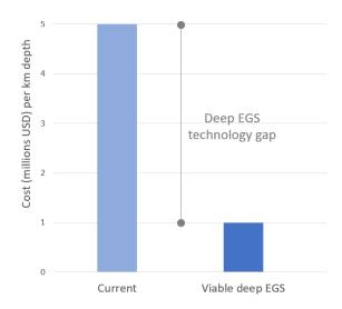
With existing drilling technologies, it is likely feasible to drill to depths of around **10 km** through hard rock at a cost between **50 and 100 million USD** per well. These costs need to be reduced by **an order of magnitude** (to 5 to 10 million USD) to make deep EGS economically viable in the current energy market.
