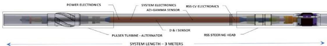
Figure 20 Picture of Hephae's high-temperature integrated MWD and RSS. (Hephae, 2024)
