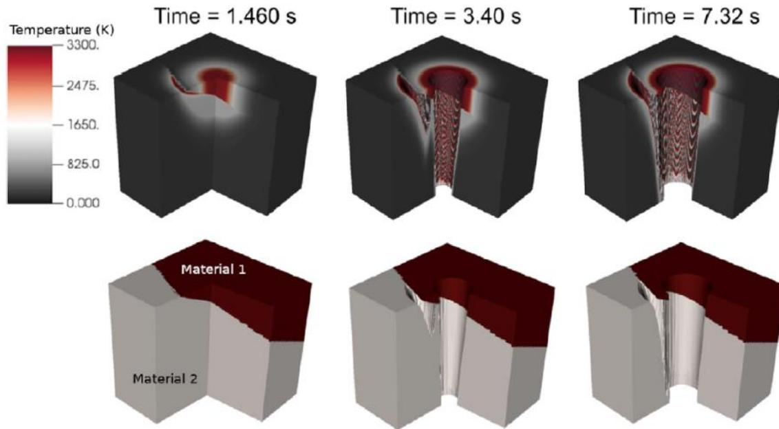
*Figure 19 Simulation results for multi-strata with heterogeneous absorptive properties, showing that the vaporization process does not produce a uniformly radial well. (Zhang et al., 2023)*
