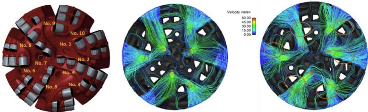
Figure 7 Nozzle configuration to optimize drill bit cooling with fluid flow
