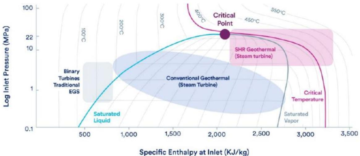
Figure 1 Specific enthalpy of pure water under increasing temperature and regimes
