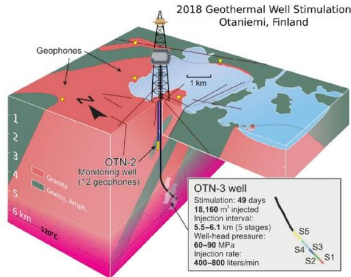
Figure 4 Geological diagram of the Otaniemi EGS site in Finland, including well location, depth, and 120°C temperature horizon. (I. T. Kukkonen et al., 2023a)
