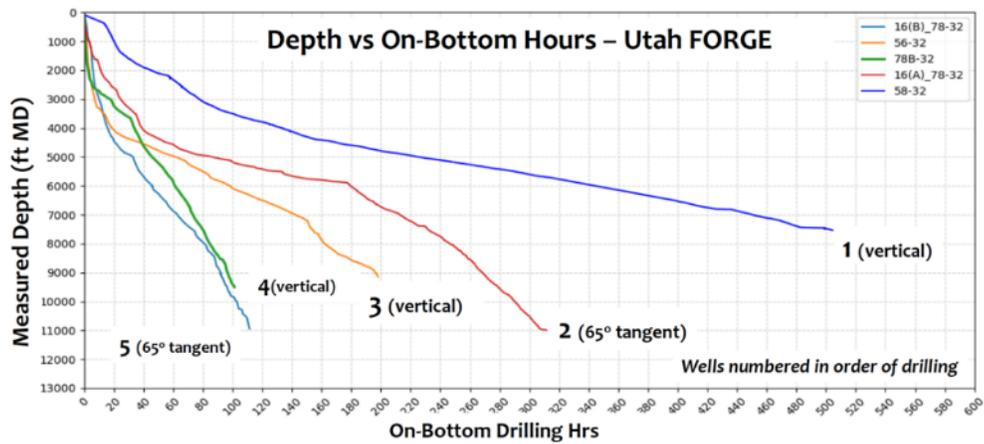
Figure 2 Depth versus on-bottom drilling hours for the wells drilled at Utah FORGE as of 2023 (Noynaert, GRC 2023)
