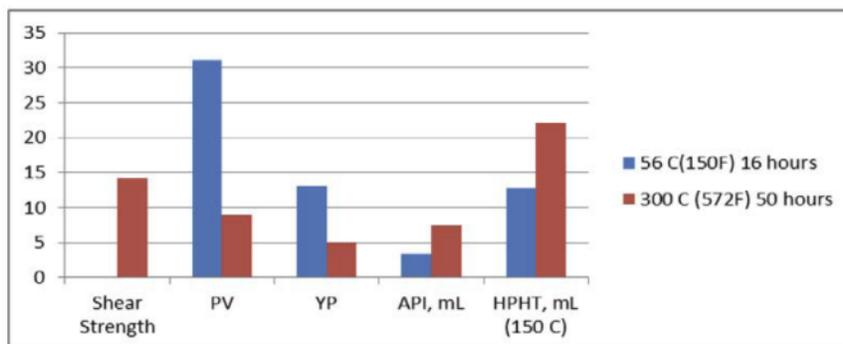
Figure 25 Drilling fluid shear strength [lbf/100ft<sup>2</sup>], plastic viscosity (PV) [cp], yield point (YP) [lbf/100ft<sup>2</sup>] after exposure to 56°C and 300°C (Stefánsson et al., 2018)
