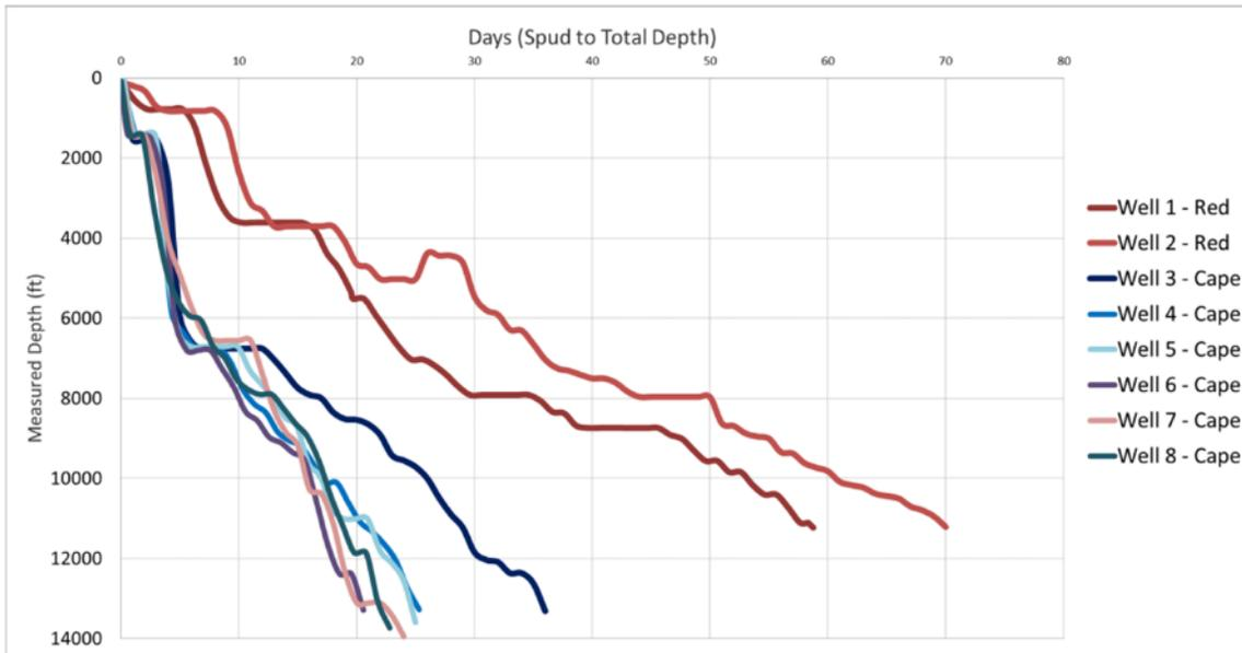
Figure 3 Total depth drilling times for the 8 wells at the Cape Station site in Utah (El-Sadi et al., 2024)
