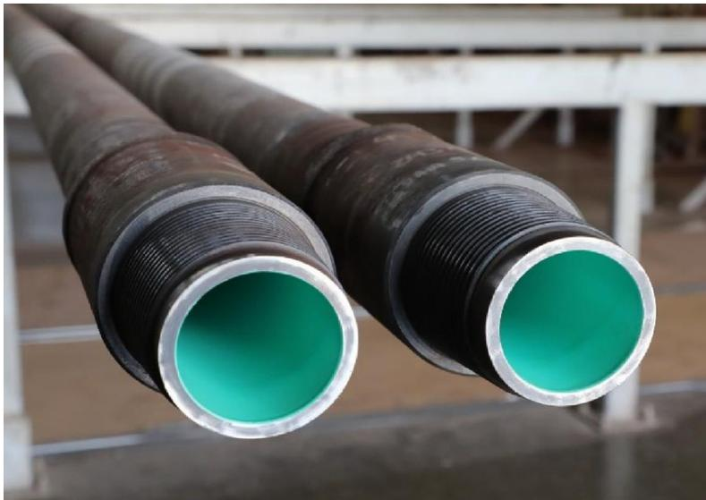
Figure 26 Low heat coefficient coating for drill pipe.
