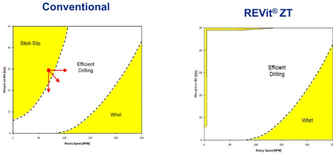
Figure 6 WOB and RPM regimes conditions for stick-slip dysfunction for conventional versus REVit® ZT drilling methods. (Nabors, 2023)
