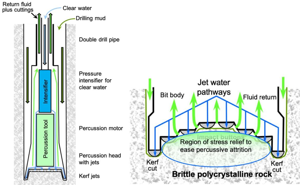
Figure 11 Orchyd and Drillstar hydro-mechanical drill system, and the bit-jet-rock interaction at the drilling interface. (Orchyd, 2023)
