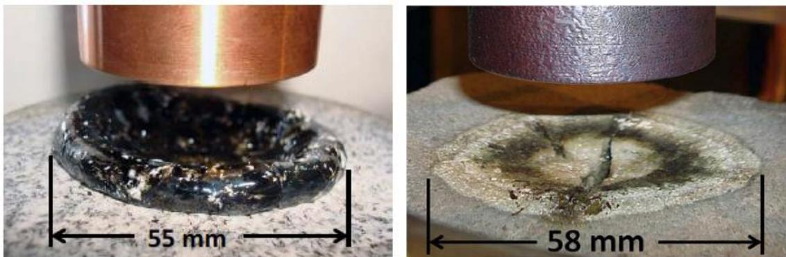
Figure 18 Ablation front, vitrified granite, stand-off distance, copper-steel waveguide (Woskov et al., 2014)
