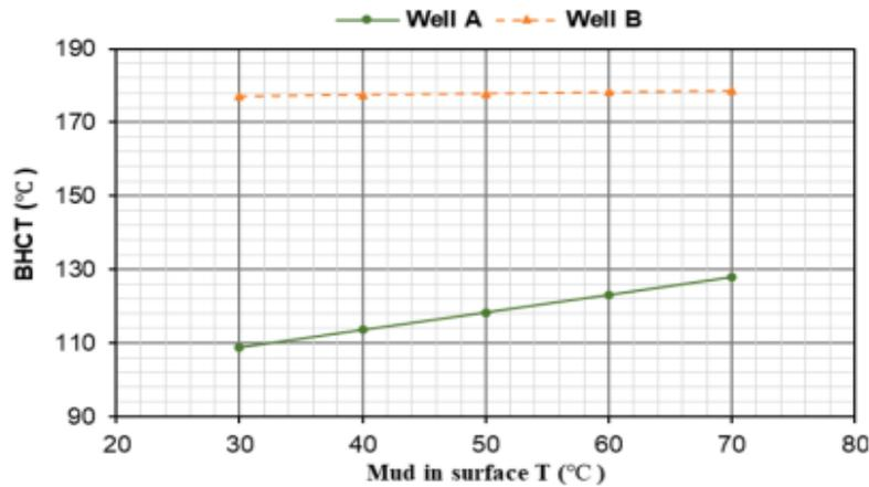
Figure 28 Impact of mud surface temperature by a mud cooler on BHCT of wells A & B. Note the reduced effect of the mud coolers action for well B (Khaled et al., 2023).
