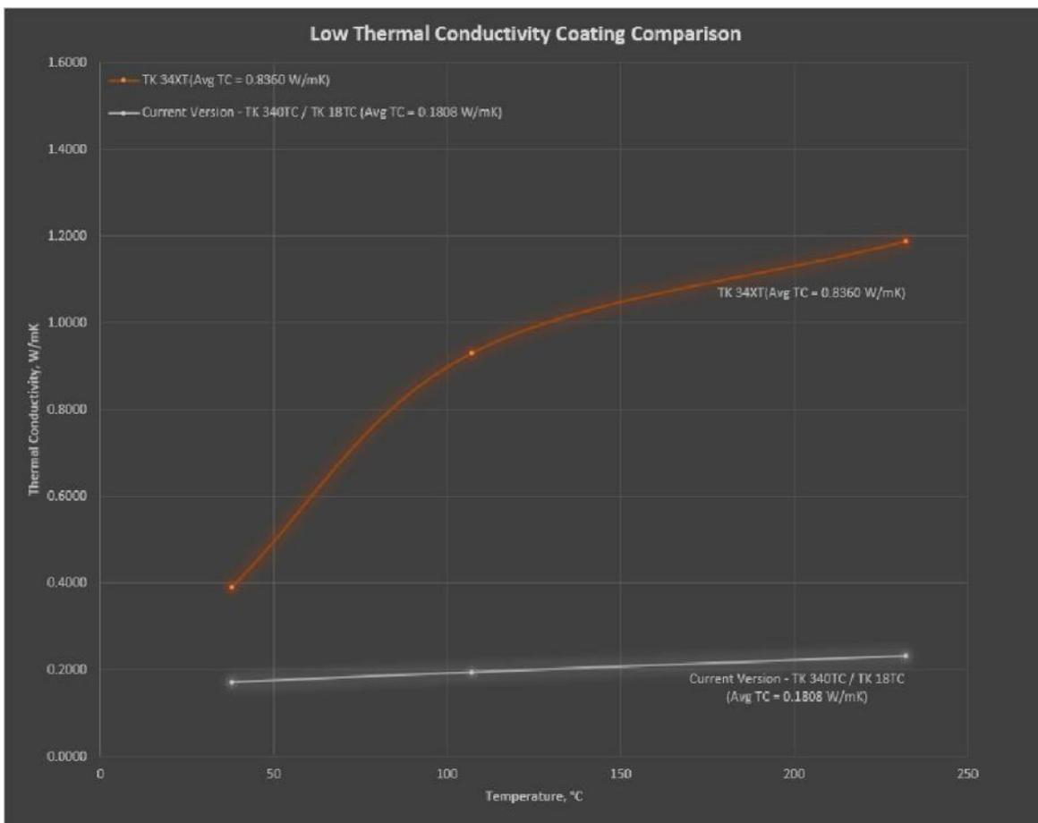
Figure 27 Thermal conductivity comparison between TK34XT and the low heat coefficient coating TK™-340TC/18TC.
