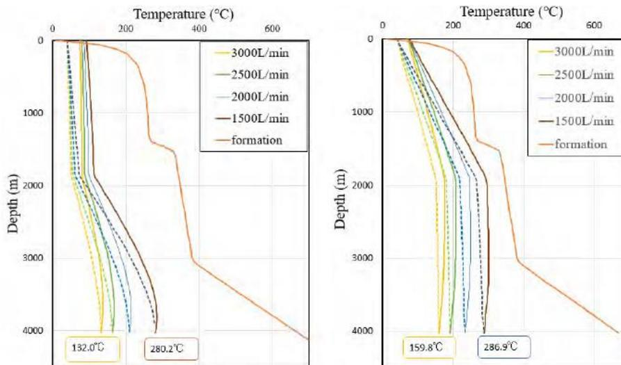
Figure 22 Temperature profiles when applying IDPs along (Left) the upper half of the wellbore and (Right) the lower half of the wellbore with drilling mud. (Ajima et al., GRC 2022)
