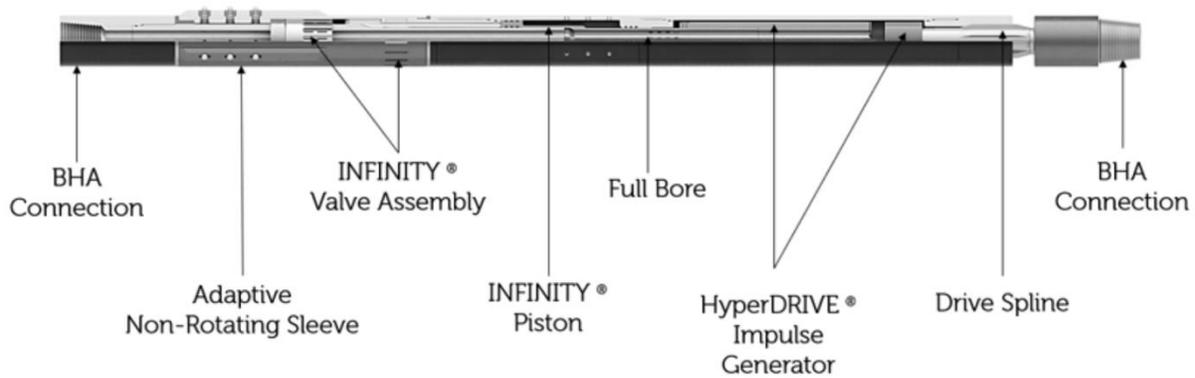
Figure 10 Schematic of the HydroVolve GeoVolve HYPERDRIVE system
