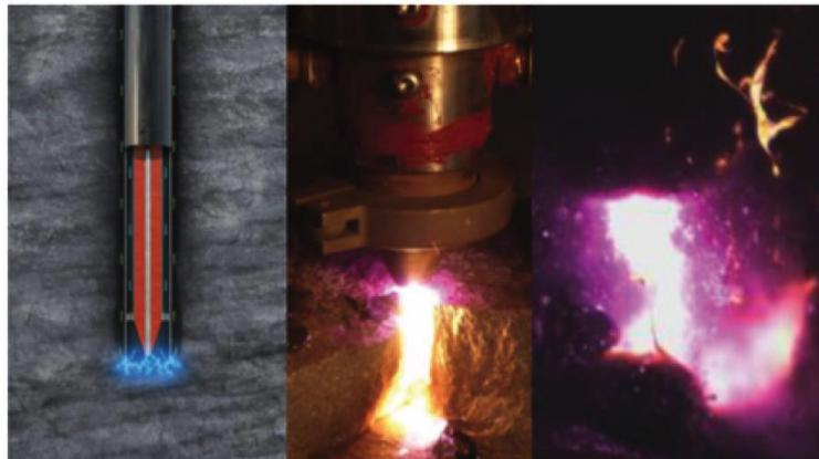
Figure 16 Schematic and real demonstration of plasma drill bit drilling through hard rock (Agrawal et al., 2016).
