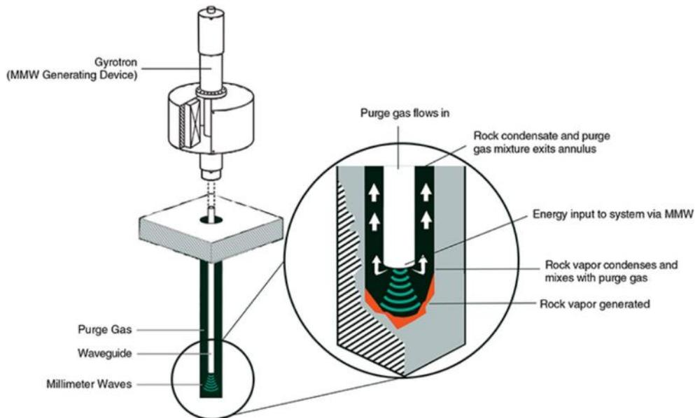
Figure 17 Simplified diagram of gyrotron-powered MMW drilling mechanism (Quaise Energy, 2023)
