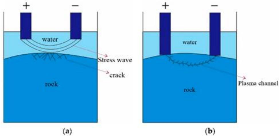
Figure 15 Visual representation of the two different versions of plasma-based fragmentation (a) non-contact-based wave formation (b) contact-based fragmentation through the formation. (Zhang et al., 2023)
