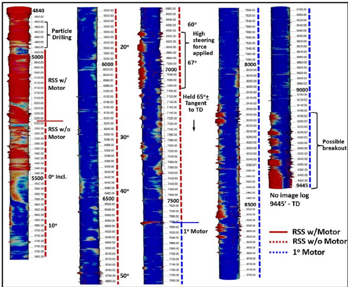
Figure 8 Profile of curved section of well 16B, showing correlations of hole smoothness and rotary-motor systems used (Noynaert, GRC 2023)
