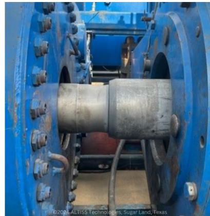
6.625" Titanium Drill Pipe Qualification Testing
